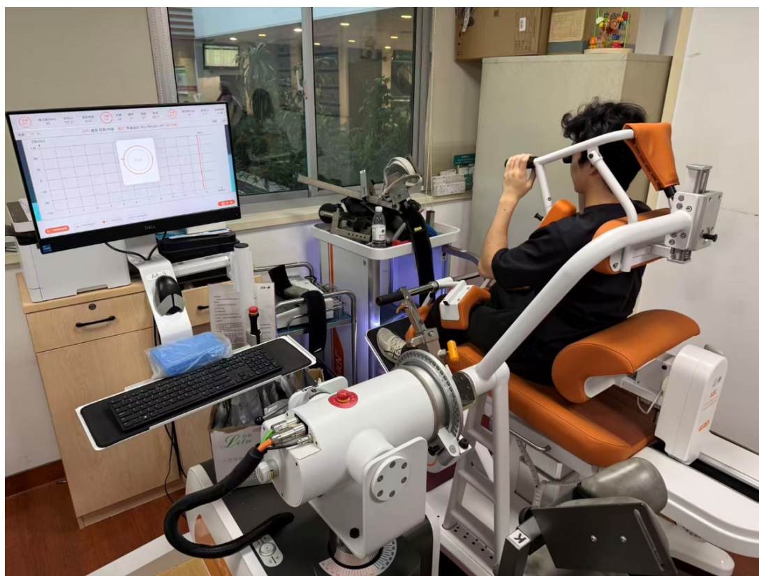
Figure 4. Isokinetic muscle strength test of the core muscle group. Participants were seated with the trunk flexion-extension axis aligned with the level of the greater trochanter. The pelvis, lower extremities, and shoulders were stabilized during testing. Isometric trunk flexion and extension strength were assessed using the IKANG multijoint muscle training and testing system.
