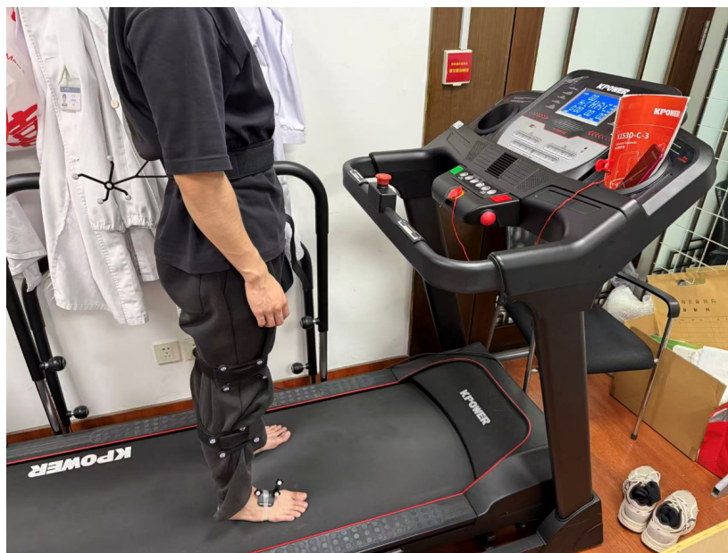
Figure 6. Plantar pressure assessment using a pressure testing platform. Participants stood and walked on the pressure testing platform to assess foot arch characteristics, inversion/eversion patterns, and plantar force distribution using the gait training and testing software.
