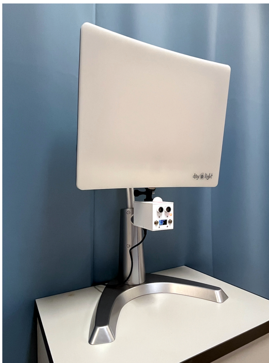
Figure 2. Light therapy lamp with monitoring sensor attached underneath.
