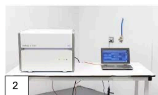
Figure 1. The Conformité Européenne In-Vitro Diagnostic (CE-IVD)-certified Mikrogen assay includes the following components: (1) Perkin elmer chemagic 360 nucleic acid extractor that uses chromagen magnetic bead technology for DNA isolation and (2) Roche LightCycler 480 for nucleic acid amplification.
