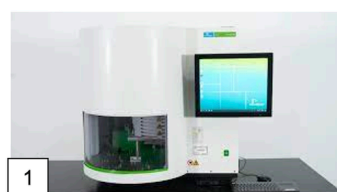
Figure 1. The Conformité Européenne In-Vitro Diagnostic (CE-IVD)-certified Mikrogen assay includes the following components: (1) Perkin elmer chemagic 360 nucleic acid extractor that uses chromagen magnetic bead technology for DNA isolation and (2) Roche LightCycler 480 for nucleic acid amplification.
