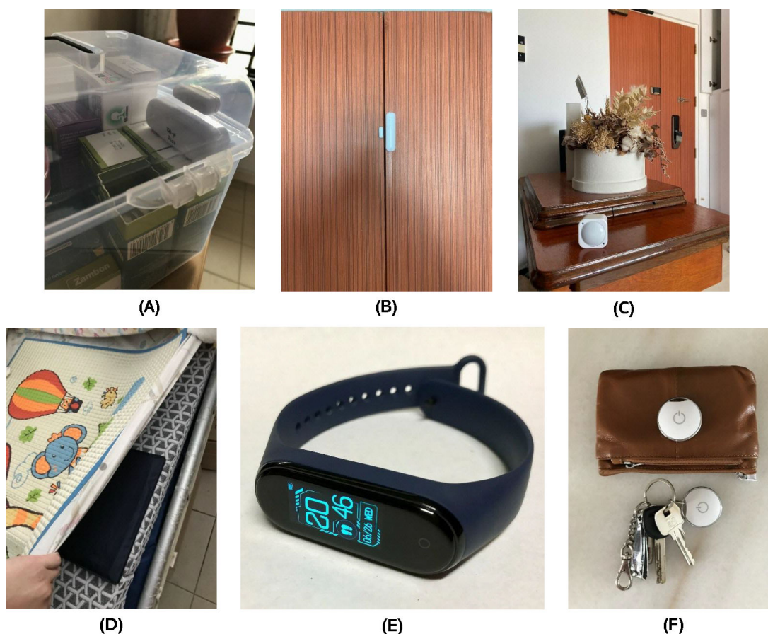
Figure 3. Home-based sensors to be deployed: (A) Contact sensors attached to the medication box. (B) Door contact sensors. (C) Passive infrared sensors. (D) Pressure sensors for beds. (E) Wearable activity band (Xiaomi Mi Band). (F) Proximity sensors on keys and wallets.
