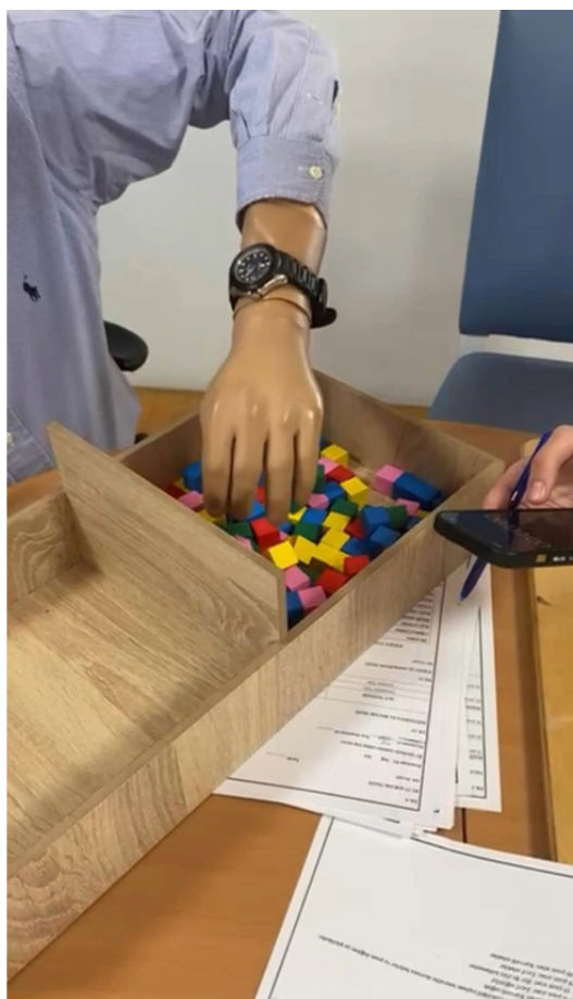
Figure 2. Box and Blocks Test in a participant who has undergone transradial amputation. The participant moves blocks between compartments within 60 seconds using the prosthetic hand.
