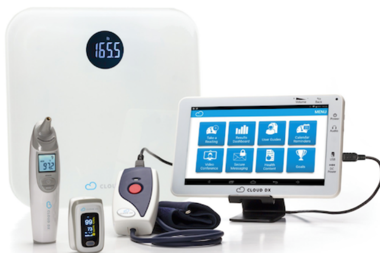
Figure 2. Cloud DX Connected Health kit. Cloud DX Connected Health kit, including Bluetooth-enabled Pulsewave wrist cuff blood pressure monitor, body weight scale, wireless oximeter, and temperature probe, paired with an Android health tablet. Reproduced with permission from Cloud DX.
