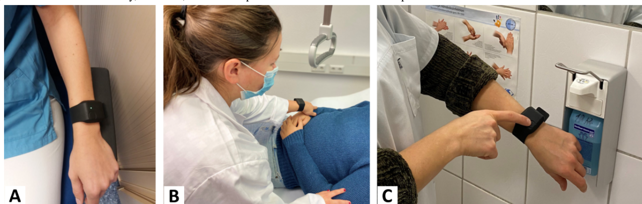
Figure 3. Electrodermal activity, heart rate, and skin temperature are recorded with the Empatica E4 research wristband.
