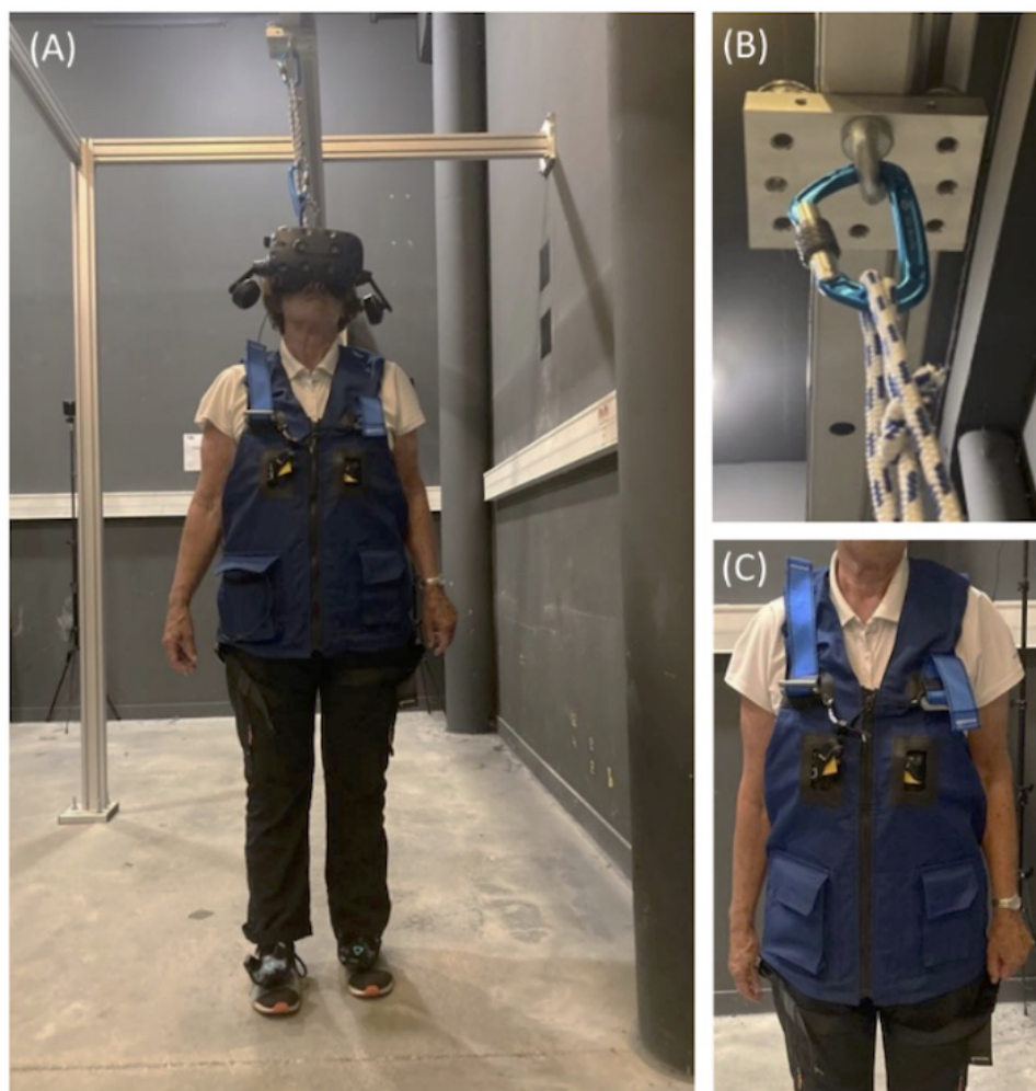
Figure 2. Test equipment. (A) A wireless HTC Vive Pro will be used to display the virtual environment. Two HTC Vive Pro 2.0 trackers will be used to record the positions of the feet and display virtual 3D shoes in the virtual environment; (B) in-ceiling rail; (C) safety harness.
