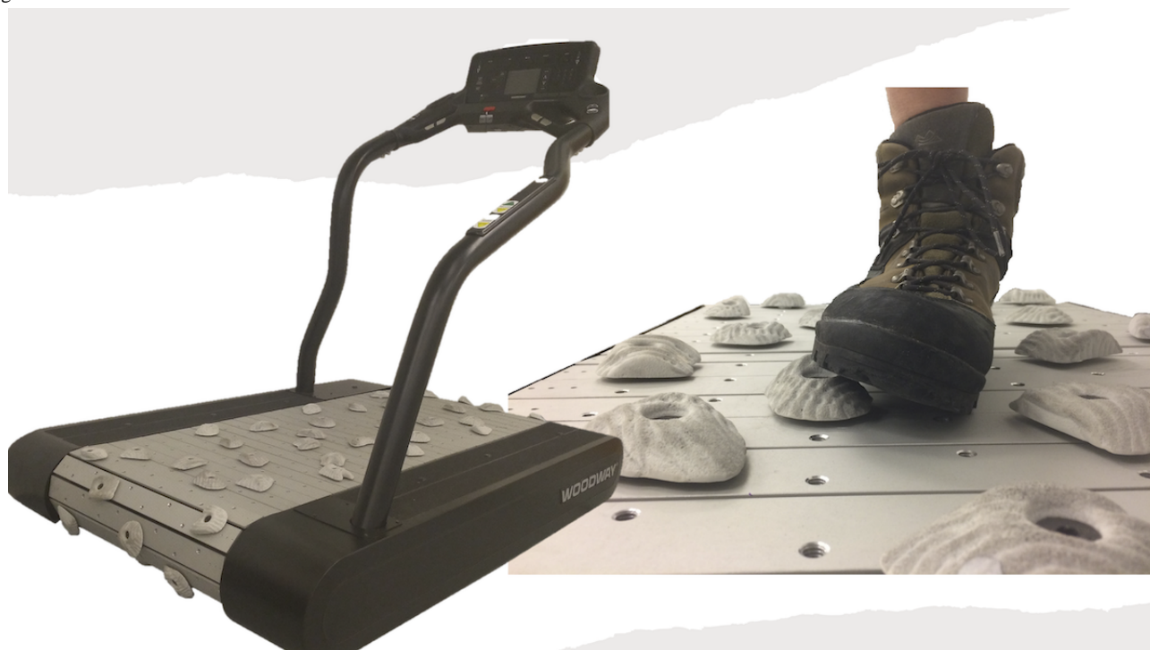
Figure 1. The custom uneven-terrain treadmill. Participants allocated to the experimental treatment will be provided a progressive gait retraining program in addition to standard rehabilitation care.
