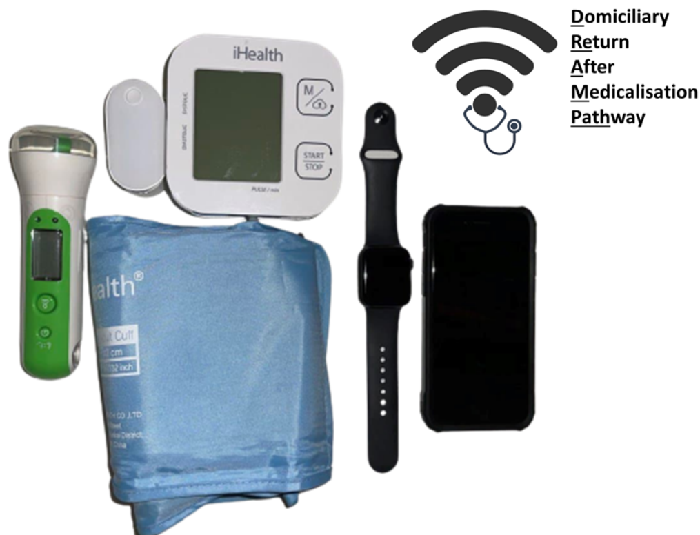
Figure 2. Smart devices issued to patients for twice-daily use: bluetooth enabled thermometer, pulse oximeter, sphygmomanometer, Apple Watch and iPhone 7 (from left to right).
