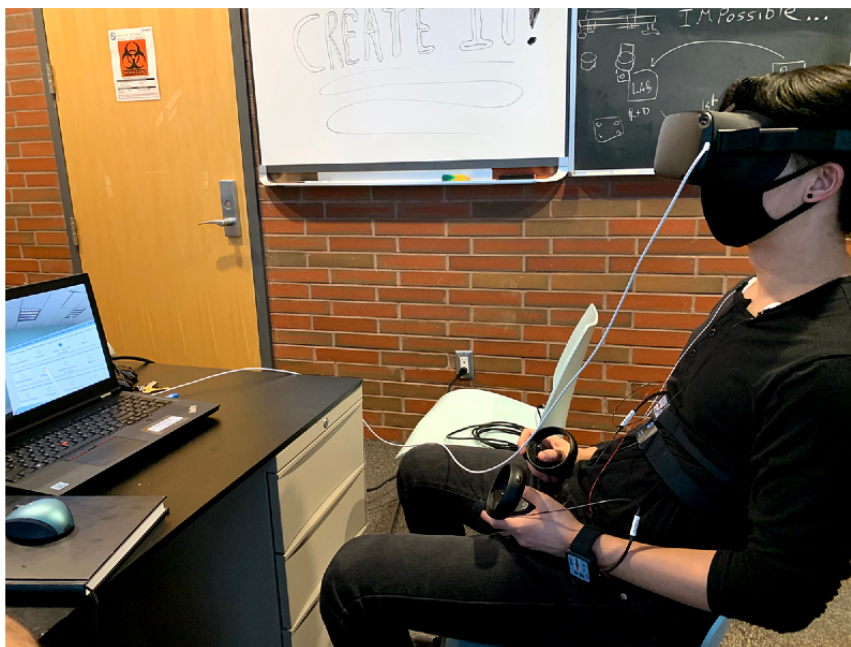
Figure 9. Example of the physical set-up: researcher wearing the head-mounted display, controllers, and Biopac sensors during the virtual reality simulation.
