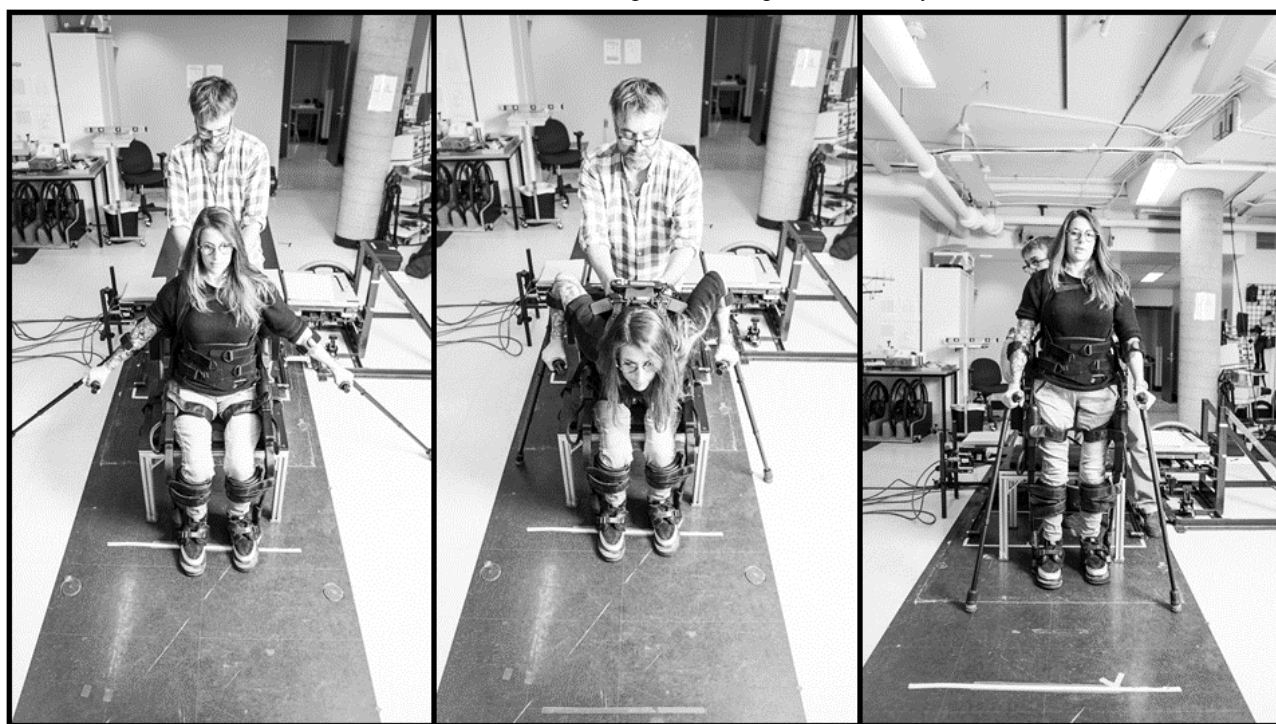
Figure 1. Wearable robotic exoskeleton for sit-stand transitions and overground walking manufactured by Ekso Bionics.
