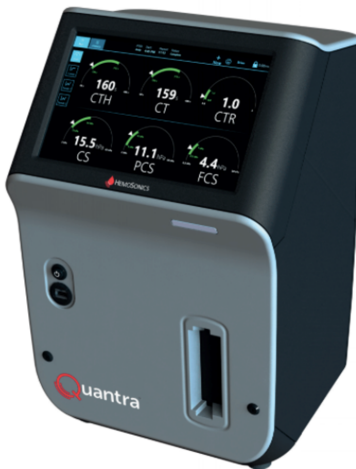
Figure 1. Quantra Analyzer. CS: clot stiffness; CT: clot time; CTH: heparinase clot time; CTR: clot time ratio; FCS: fibrinogen contributions to clot stiffness; PCS: platelet contributions to clot stiffness.
