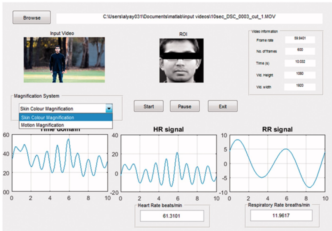
Figure 1. MATLAB graphic panel of the proposed system. HR: heart rate; RR: respiratory rate.
