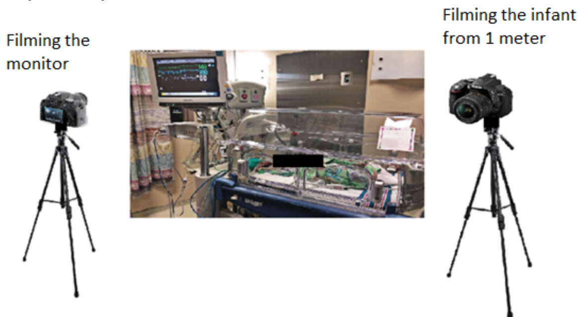
Figure 2. The experimental set-up for data collection.
