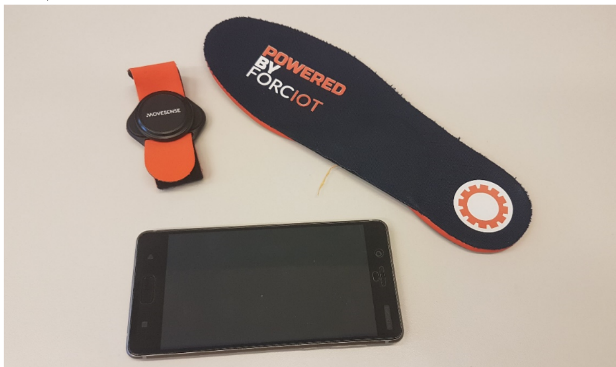
Figure 2. Sensors used in the study: Movesense smart sensor (upper left corner), Forciot smart insole (upper right corner), and Nokia 6 smartphone (lower left corner).
