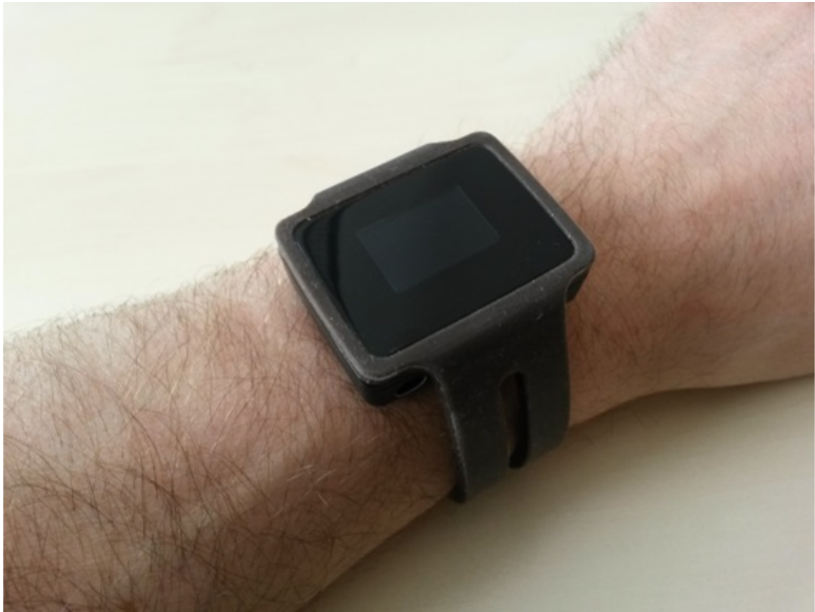
Figure 3. Sensor bracelet developed for insideDEM.
